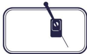
When locomotive power is cut, pneumatic wipers often come to rest in a position that blocks the forward facing camera
