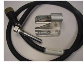
Traction Motor Sensor w/two-piece design
